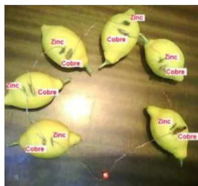
Image 1: Example of assembly with 6 lemons
