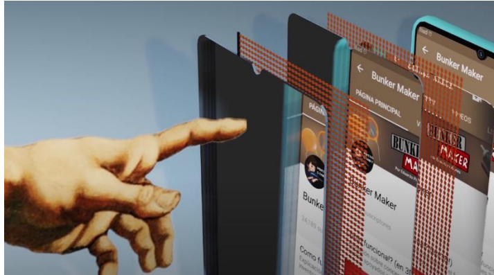
Image 1: Representation of a telephone screen. The copper grids are the electrodes, and in between is the insulator.
