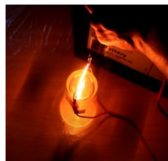
Image 1: Graphite bar emitting light when the electric current passes.
